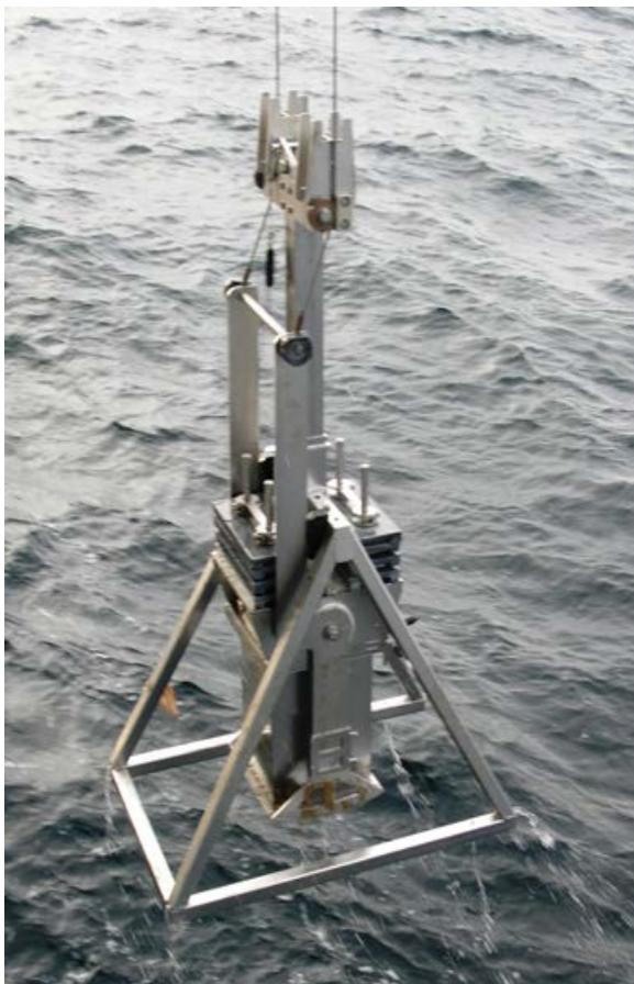
Figure 2. Boxcorer being recovered.
