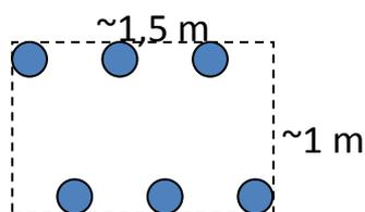
Figure 1. Photo showing the multicorer on deck after sampling. Drawing showing dimensions and placement for the 6 cores.
