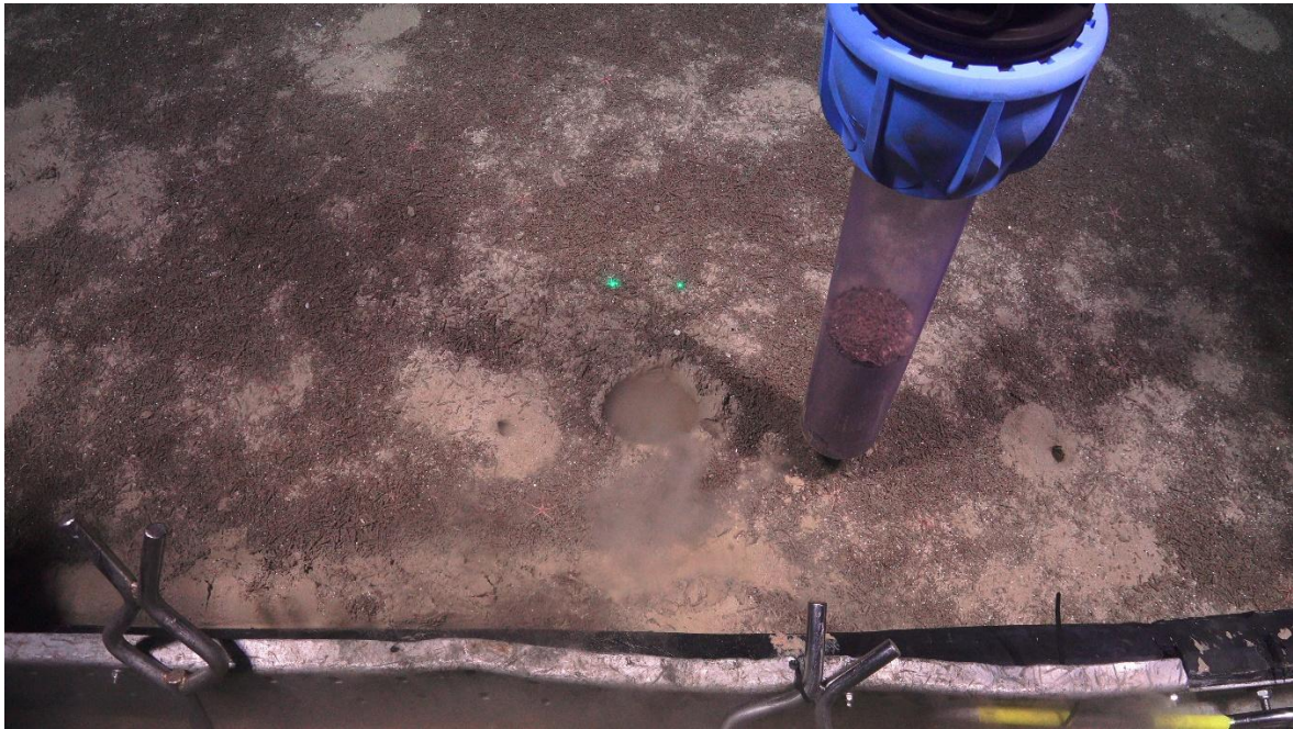
Figure 1: Sediment core sampling with an ROV-operated push corer system.
