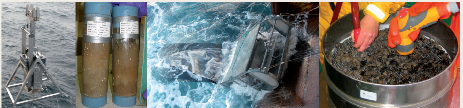
A box corer (left) samples sediment data and the RP sledge (center) collects data on benthic fauna. Cleaning of samples for benthic analysis (right).
