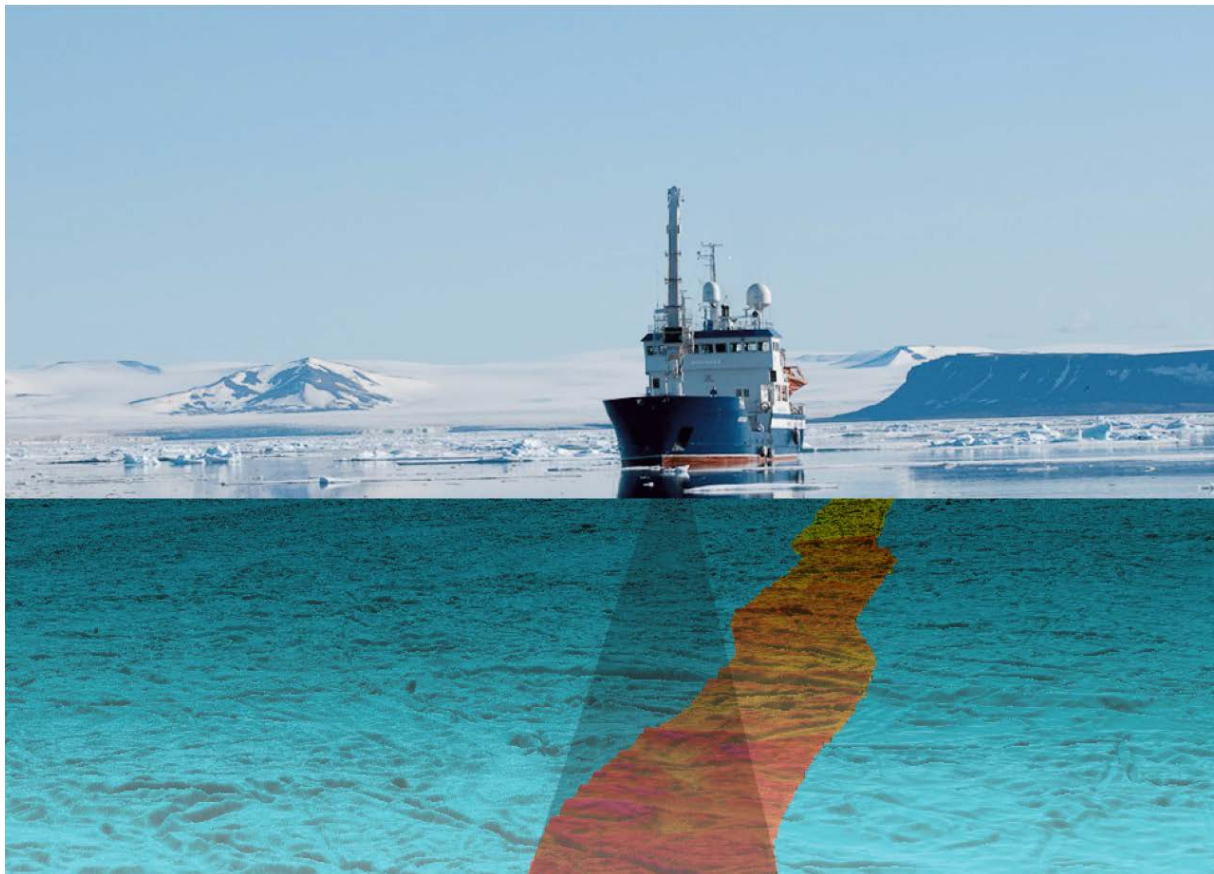
Figure 1. Illustration of surveying using multibeam echosounder.
